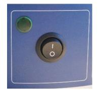
The main switch of the tissue floating bath must be **off** (position O).
