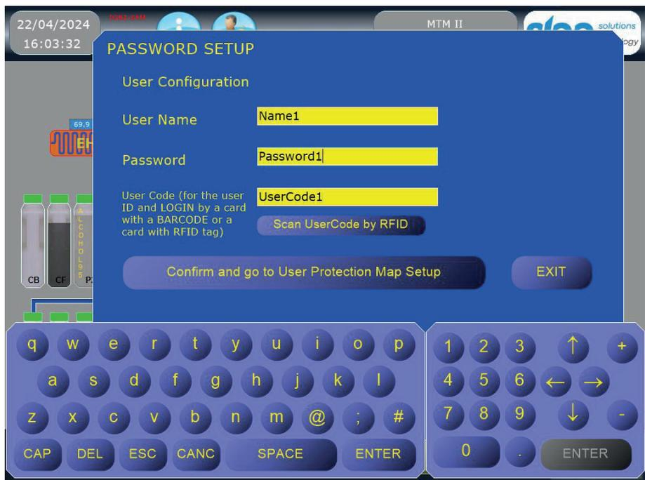
The operator's credentials are assigned on this page. Each operator must be identified with Name, Password.
