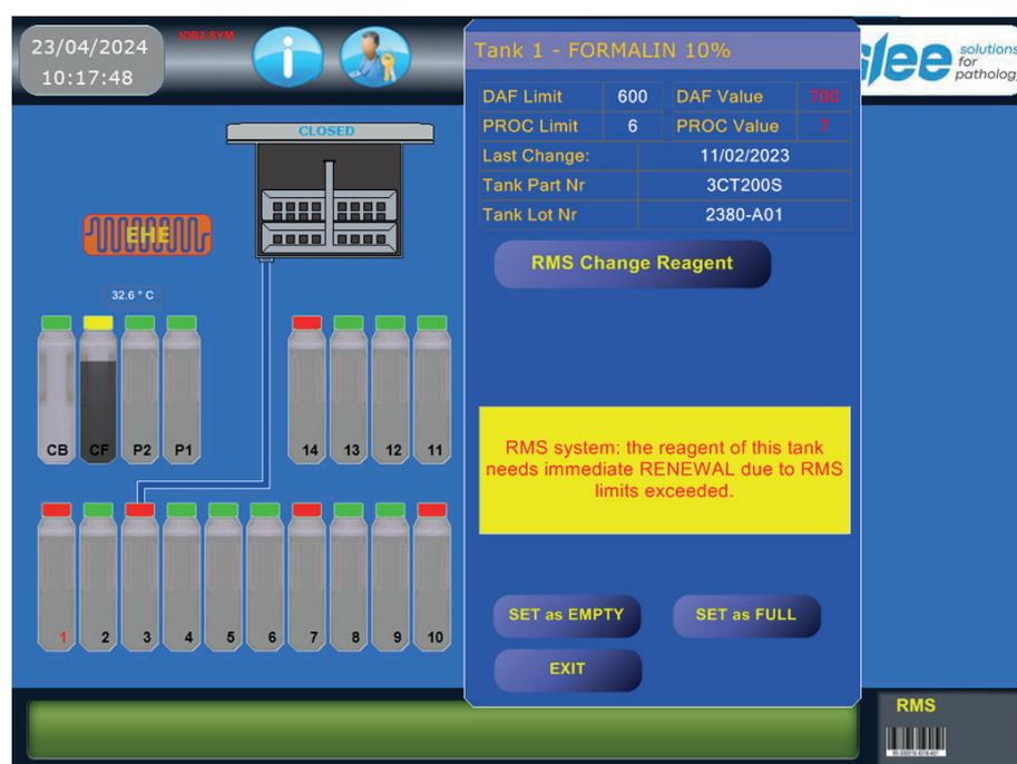
By clicking on the "RMS Change Reagent" button, the reagent is replaced and to guide the operator, 2 fields TANK OUT and TANK IN are displayed.
