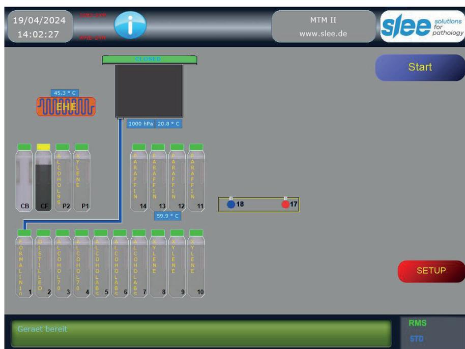
At the top left, near the clock, there is an icon with the letter "i", by pressing this a temporary window appears (which closes automatically after 30 seconds) containing information on the most important parameters regarding the status of the device:
