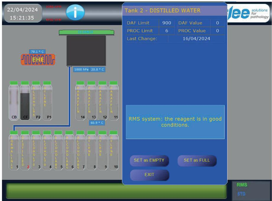
If you want to replace a reagent tank whose cap is green, (considered in good condition by the RMS system: DAF value < DAF limit).It is necessary to press the "Declare empty" button, the tank cap will be displayed in Black.
