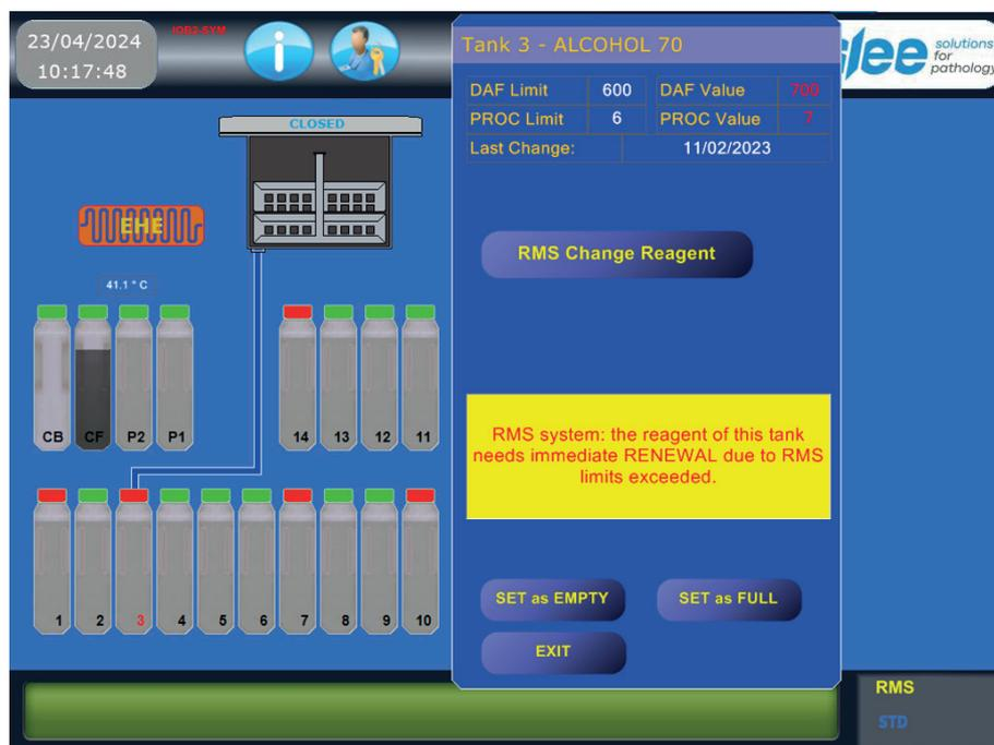
If the DAF Value or the number of Processes has been exceeded, the "RMS Change Reagent" button is displayed.
