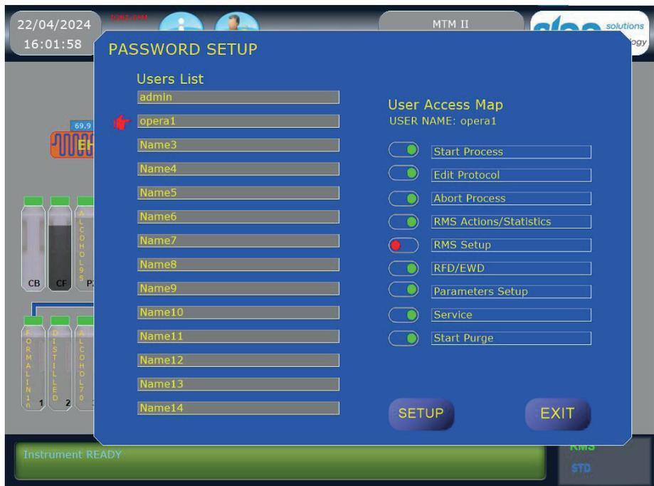
There are nine functions that can be protected and the laboratory manager (administrator) must decide which functions to protect based on real security needs.
