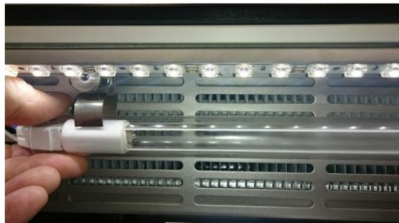
The connector can be plugged into two directions of polarity, a switch is excluded.
