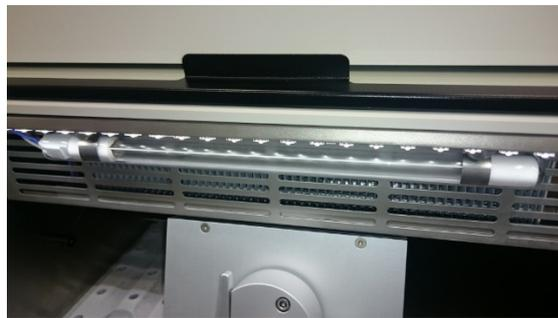
Once the plug is connected to the UV- Lamp, the final step can be done now and the UV-Lamp unit can clip into the retaining clips.
