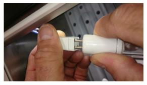
The connector can be plugged into two directions of polarity, a switch is excluded.
