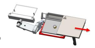
After removing the blade, pull out the lever, remove the pressure plate and clean the blade holder with a brush or cloth.
