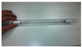
Slide the UV lamp as shown into the glass bulb. Keep 2 cm space before the end position will be reached, this place will be needed to connect the UV Lamp with the connecting plug. (Pic. 2 & 3)
