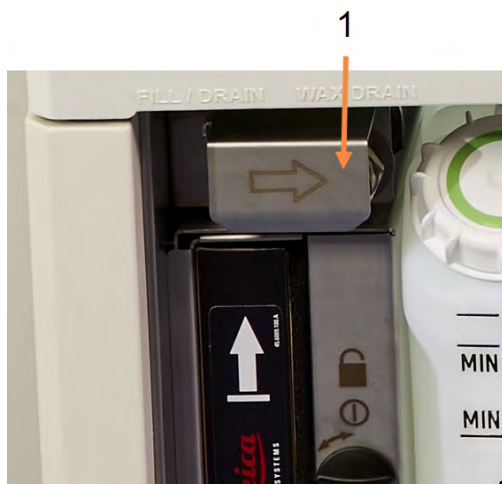
Figure 5-11: Remote fill/drain flap open with reagent line (left) and wax waste line (right)
