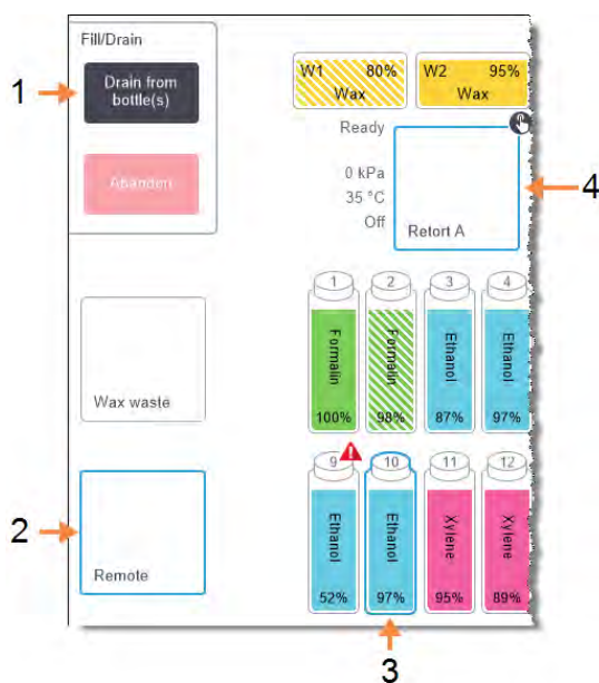
Figure 5-13: Remote fill/drain setup for draining bottles
