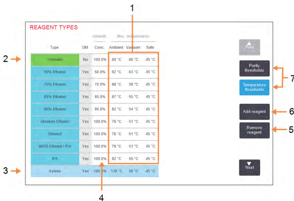
Figure 5-3: Reagent Types screen, temperature thresholds view, using recommended reagent types for xylene-free processing
