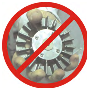
Figure 7-9: Stirrer handling—correct (left) and incorrect (right)
